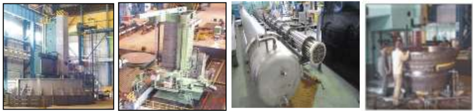
16 m Dia. Vertical Lathe 12 m Boring & Milling Machine Heat Exchangers/ Air Coolers Turbine Blade Carrier
